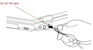
Figure 1-3 Connecting the adaptor to the computer
